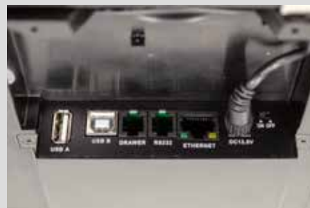
Connections: USB-A, USB-B, cash drawer (DRAWER), RS232, Ethernet, Power supply, ON/OFF
