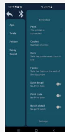
Here you can set important parameters such as scale type, communication protocol, customer, product and batch visibility, and pre-programmed tare management. This area also offers options to configure the linked printer and to adjust ticket printing details.
